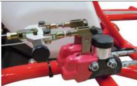
Front and Rear Combination Foot brake Master Cylinder (Open system)
