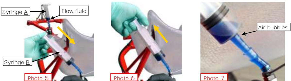
10. Slowly operate the brake pedal about 2 to 3 times. If still Air remains in the master cylinder, the bubbles will rise up through the port into the syringe **A**. (photo 8)
