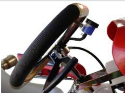
Front Hand brake Master Cylinder (Open system)
