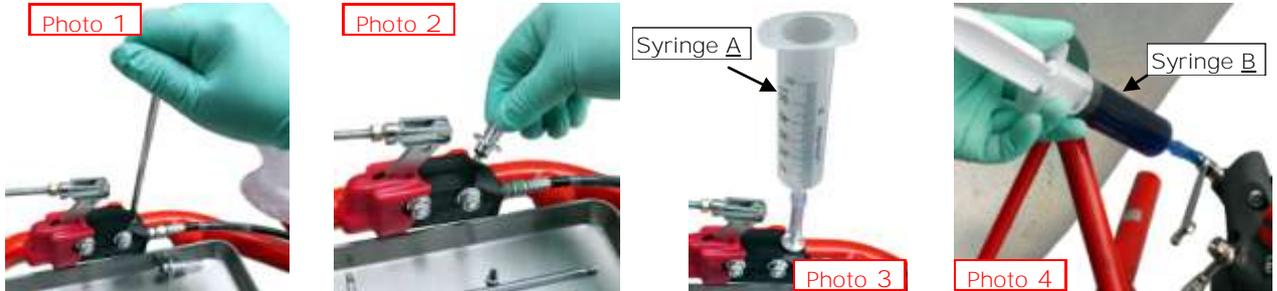
5. Loosen the bleed nipple by 1/2 of a turn to open it.
