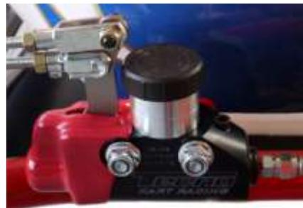
Rear Foot brake Master Cylinder (Open system)
