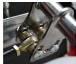
Tie rods fixation on steering column
