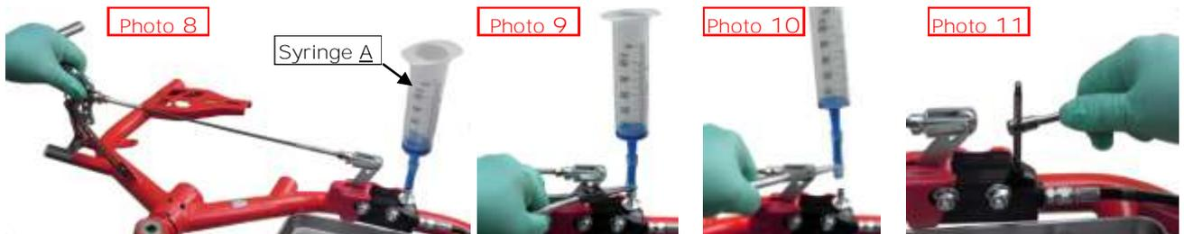
14. Operate the lever of the master cylinder. The lever must be stiff and not have the play. If no, repeat step 1 to 12.
