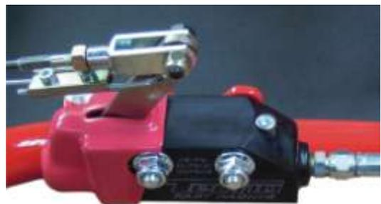
Rear Foot brake Master Cylinder (Closed system)
